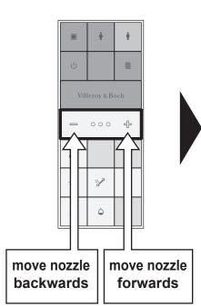
Press – or + as many times as necessary to achieve the desired nozzle position.
