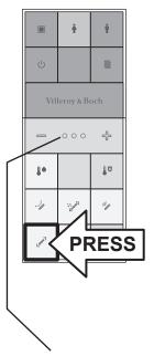
The LEDs show on which position the nozzle is set.
