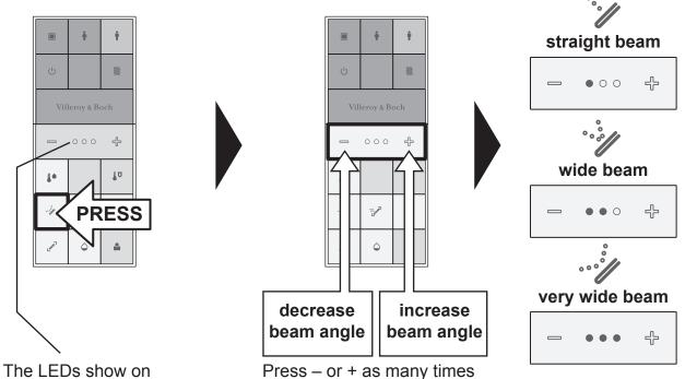
Press – or + as many times as necessary to achieve the desired beam angle.
