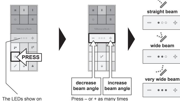
Press – or + as many times as necessary to achieve the desired beam angle.
